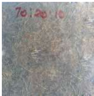
Fig 4 75% of epoxy resin 15% of coir fiber 10% of fly ash(75 micron)
