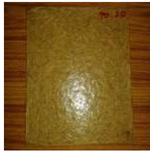
Fig2 75% of epoxy resin 25% of coir fiber
