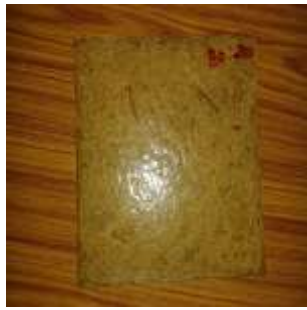
Fig1 80% of epoxy resin 20% of coir fiber
