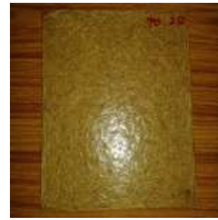
Fig3 70% of epoxy resin 30% of coir fiber
