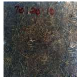
Fig 6 70% of epoxy resin 20% of coir fiber 10% of fly ash(75 micron)
